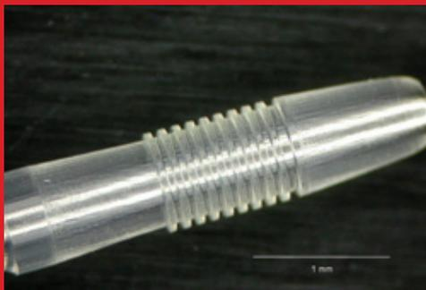
**Figure 3: Polymer implant produced using 3D laser micromachining techniques. Lasers allow microfabrication beyond the capabilities of CNC machining.**
