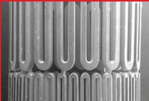
**Figure 4: Bioabsorbable stent machined using UV laser micromachining technology. Use of UV photons is key to avoiding alteration of polymer properties from thermal effects.**
