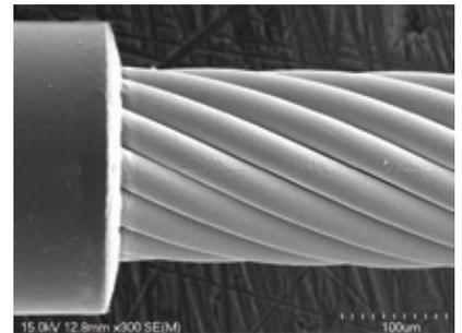
**Figure 5: Laser stripped implant lead. Insulation can be cleanly and precisely removed without damage to fine wire filars.**
