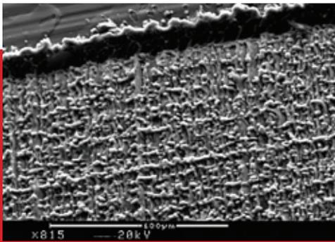
**Figure 1: Laser textured titanium alloy surface. Micro to nano scale morphology can be achieved in a clean, non-contact process.**
