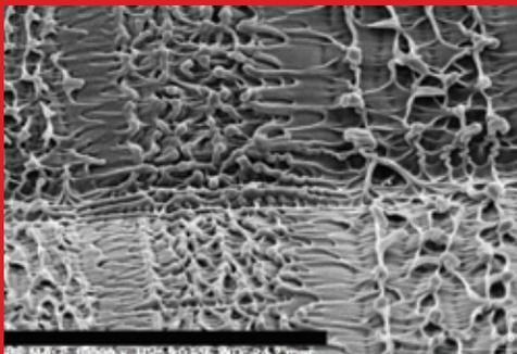
**Figure 2: Laser textured polymer surface. Micro to nano scale morphology can be produced in a wide range of polymers.**
