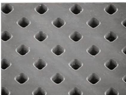
Polymer-based embolic protection filters have thousands of laser-drilled perfusion openings that enable blood flow while also capturing emboli.
